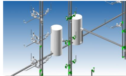
S4 – Fig 129 : Sanitary System
