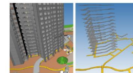
Accessible Route within BIM model (left) and with rest of BIM model hidden (right)
